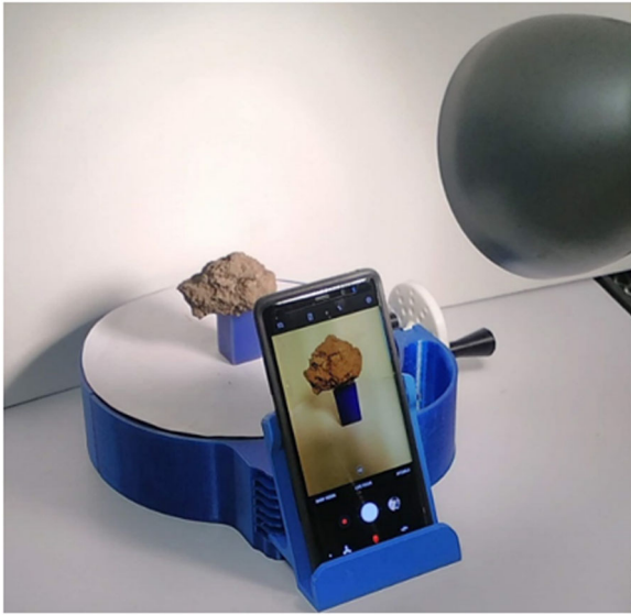
FIGURE 1 Experimental setup of 3D printed turntable with mobile phone ( https://www.thingiverse.com/thing:1762299 ). Each soil ped was shaved flat on one side and was placed on the blue plastic rectangular sample stand. The sample was then rotated 360 degrees and thirty-five overlapping photos were taken as the sample rotated in front of the camera. The table lamp was used to provide consistent illumination. White paper was placed under the sample stand and white poster board was used as a backdrop to avoid artifacts in the photogrammetric 3D render.
